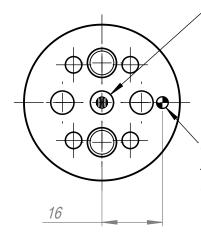
6<sub>mm</sub> Slotted Spring Pin 5.5mm Max protrusion from surface
